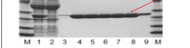
Figure 10. Purification of TEV protease from expression vector pMHT238Δ in BL21-CodonPlus-RLP1 strain (Blommel and Fox, 2007). TEV protease purification employs two-step procedure consisting of IMAC followed by cation exchange chromatography. The average yield is 15 mg of purified TEV protease obtained per gram of cell paste.
